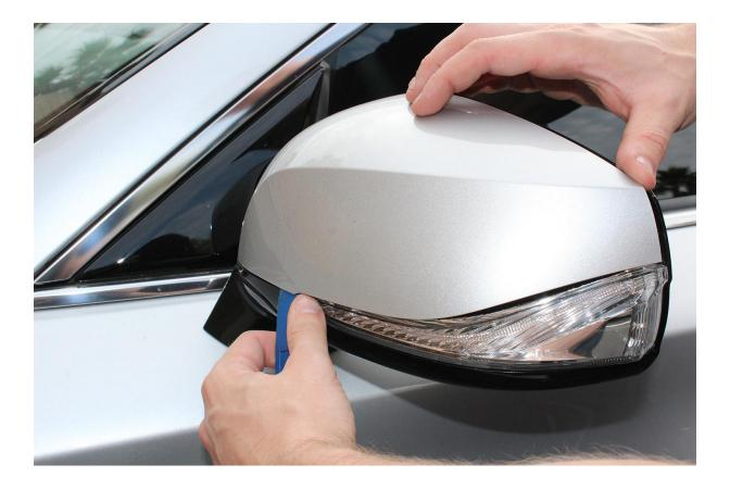
7. As you work your way around, the mirror will try to hang on at the closest point to the car. Continue to apply force pushing the cover towards the front of the car, and avoid allowing the cover to "hinge" at this point, as that may cause damage to the clips on the original cover. If necessary, you can also fold the mirror body in to get another angle on the inner-most clip.
