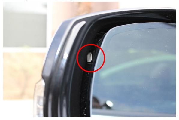
2. Using a screwdriver or plastic tool, push this tab (It will bow slightly towards the car).
