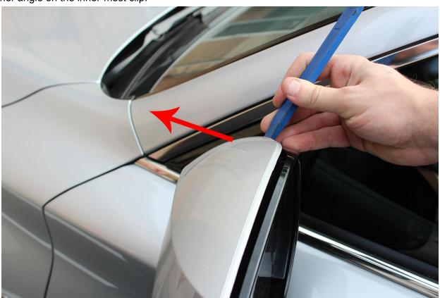
8. Eventually, the cover will give up. You can see the 6 clips holding it in place here. The far left on is the one we push at the very beginning of the process.
