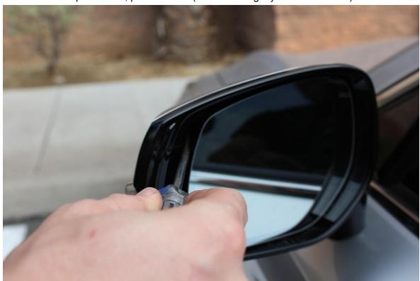
3. While you push that tab, start working a thin plastic tool in between the outer housing and the frame around the mirror, starting near the end of the turn signal lens.
