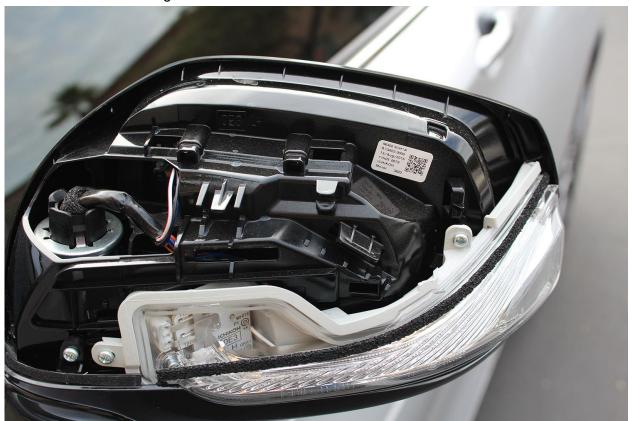
10. Finally, just line up the clips on the new cover with the receiver holes on the body and push towards the mirror housing (applying force towards the back of the car). It will pop into place, and that's it!
